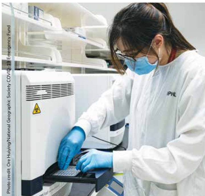
Loading of sample strips into a Real-Time PCR System
