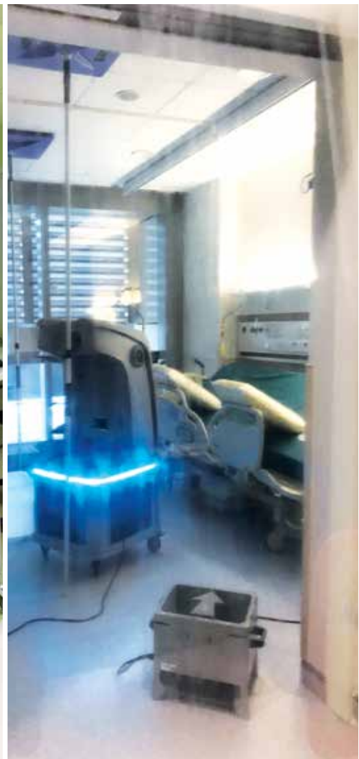
Hydrogen Peroxide Vapour decontamination of patient room
